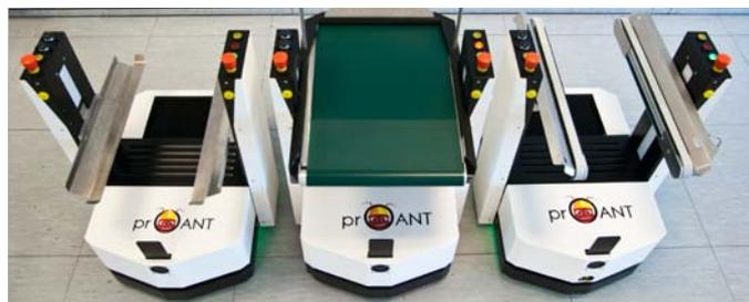
Transfer of load can be realized with every conveyance technique. Depending on load handling and demand very different active and passive transfer stations can be designed for example simple Pick & Drop Stations at work stations.
