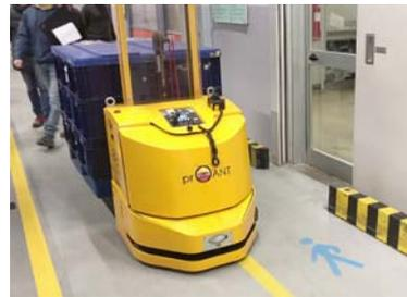
The proANT 576 is safe for people and equipped with safety laser scanners all around. Light sensors on the forks ensure that the pallets are safely picked up, and switches monitor the correct position during pick-up and transport.
