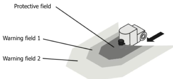
Figure 3: proANT aAGV's protective and safety fields
