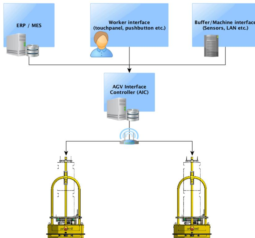
Figure 5: Transport information flow using AGV Interface Controller (AIC)
