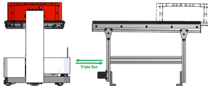
Figure 4: Hardware handshake using triple eye (handshake not yet reached)
