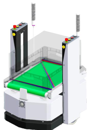
Figure 7: Active conveyor on proANT aAGV
